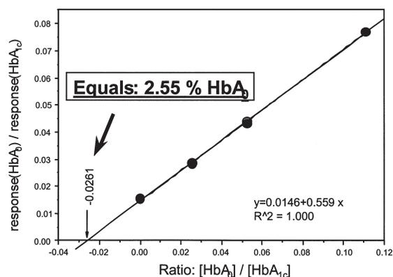
**Figure 13** Determination of the amount of HbA<sub>1c</sub> preparation by standard addition procedure.
