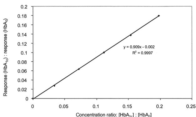
Figure 7 Calibration function for the HPLC-CE approach.
