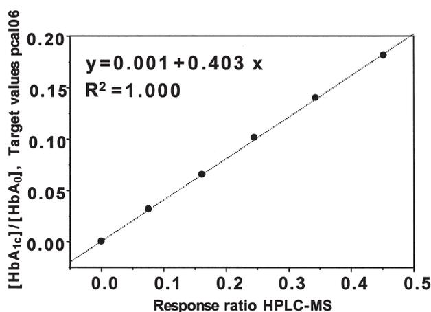
Figure 6 Calibration function for HPLC-ESI/MS.
