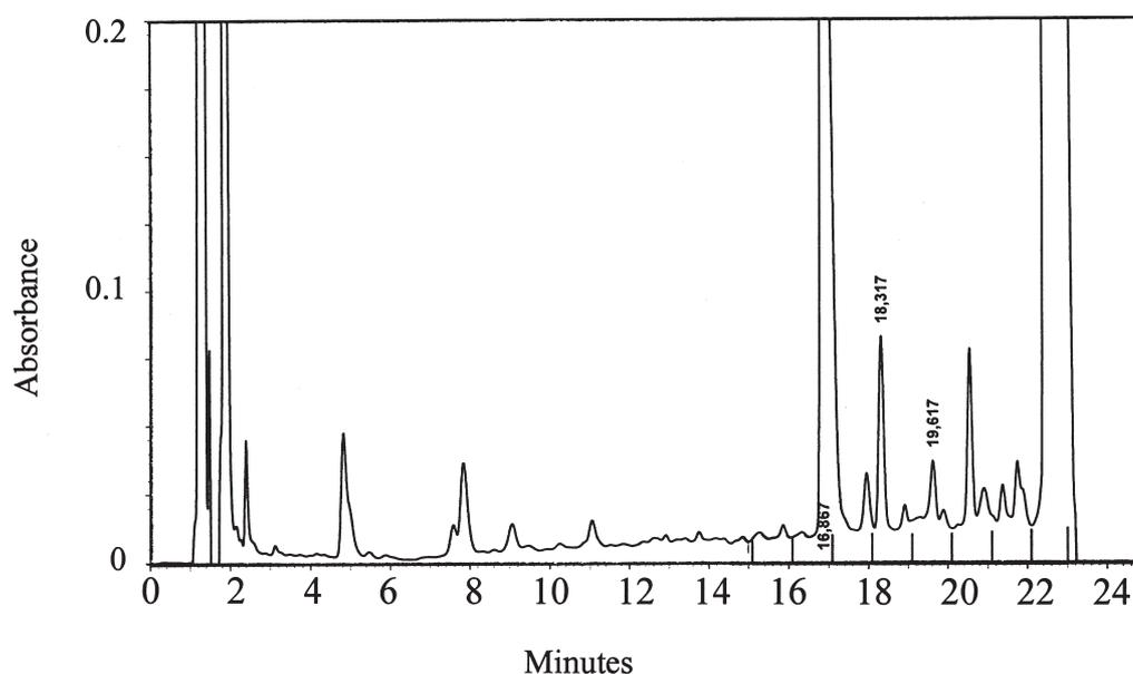
Figure 8 HPLC-C<sub>18</sub> chromatogram of a mixture of peptides from proteolytic digestion of haemoglobin chains. Fractions 16–18 min are collected for capillary electrophoresis.
